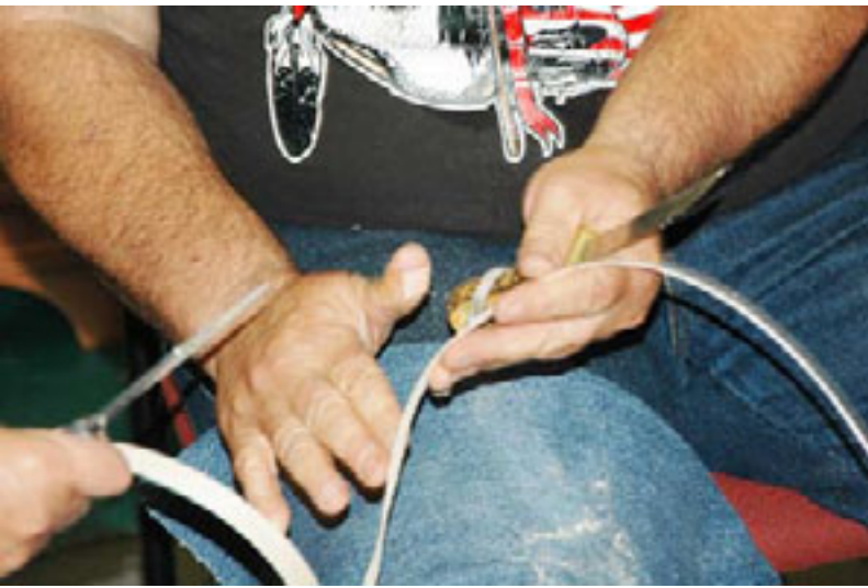
Once you have a strip you want to use, you must shave it along the grain until it is smooth.
