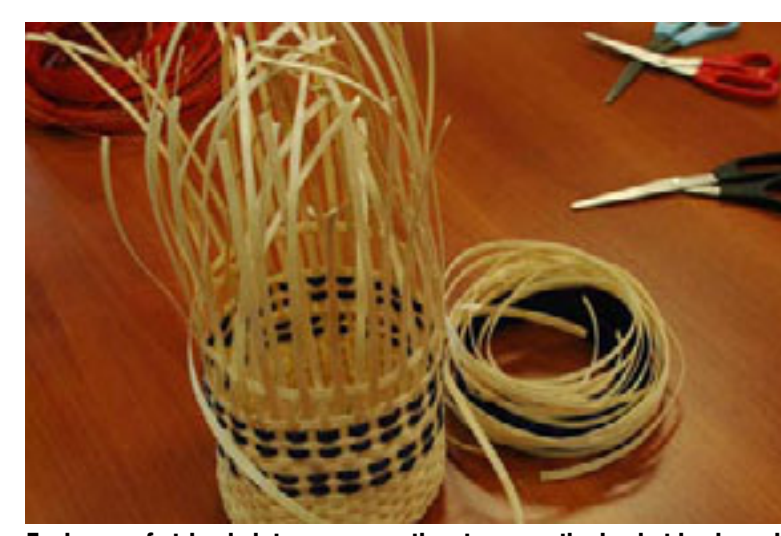
Each row of strips is interwoven on the staves as the basket is shaped.
