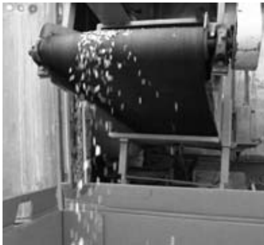
Tokens are chopped in the semi. Chipped pieces of the destroyed tokens are put on the conveyer belt and put into boxes.
