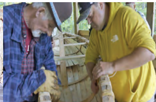
Inserting the ribs.
