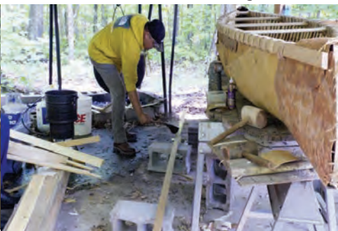
Heating the top gunnel.
