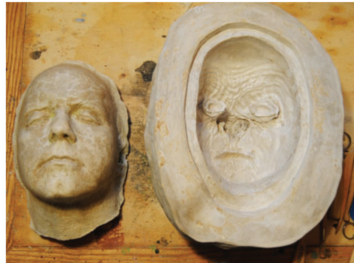
Face cast and mold. Once the foam latex is poured into the mold (right) the face cast (left) is pressed into the back of it so that the finished mask fits over the wearers face.
