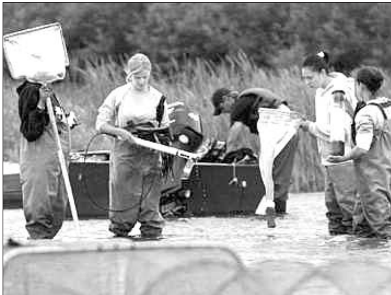
Team members collect aquatic insect samples and use a multi-probe meter to measure water quality. A mini-fyke net in the foreground catches fish.
